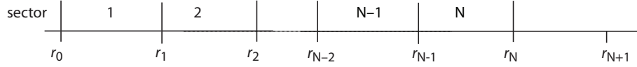
FIG. 14. Schematic partition of the r -axis into a series of sectors. The last sector ends at r = r_N . To determine the log-derivative matrix at r = r_N , we need to propagate one more step, out to r = r_N + h .
